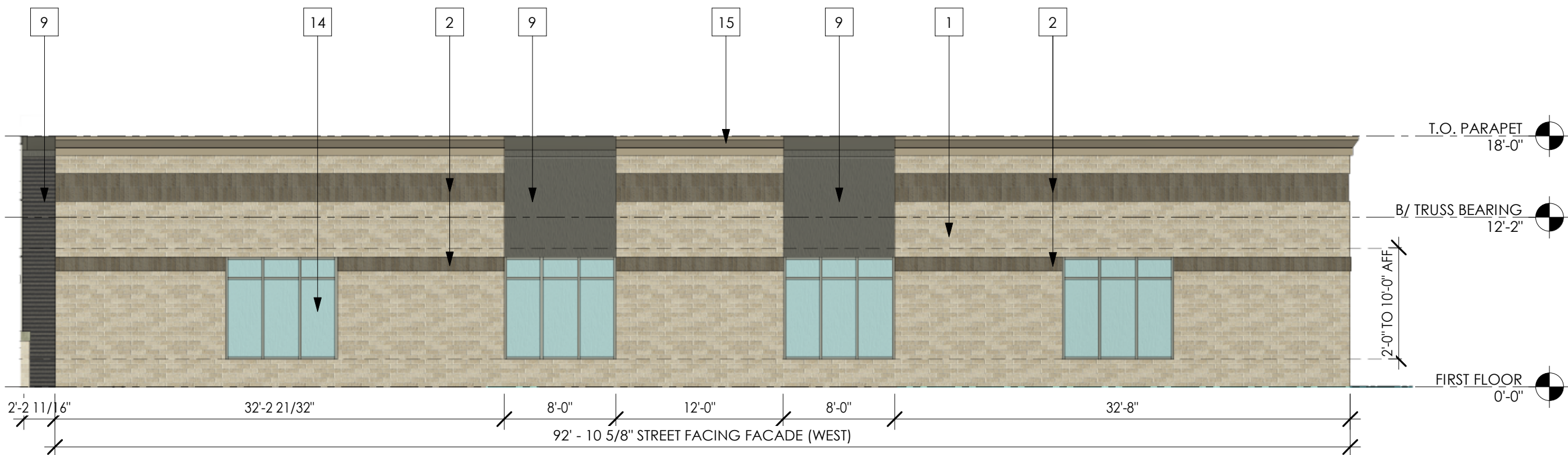
8S PARTIAL WEST ELEVATION (SOUTH) RD-1.2C SCALE: 1/8" = 1'-0"
