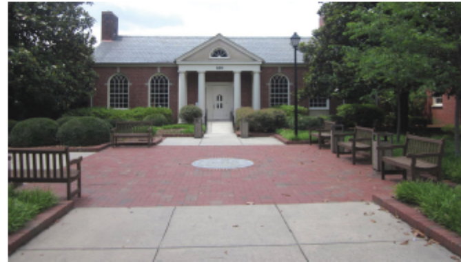
The basketweave brick pattern of this plaza reflects the traditional vocabulary of the district. The accessible ramp is subtle and serves as the main route to the building entry.
