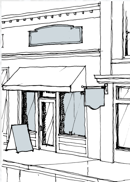
Appropriate signage locations for historic commercial buildings
