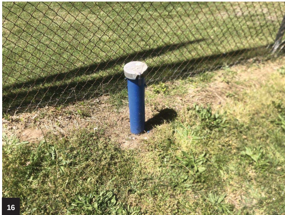
Monitoring well near northeast corner of baseball diamond
