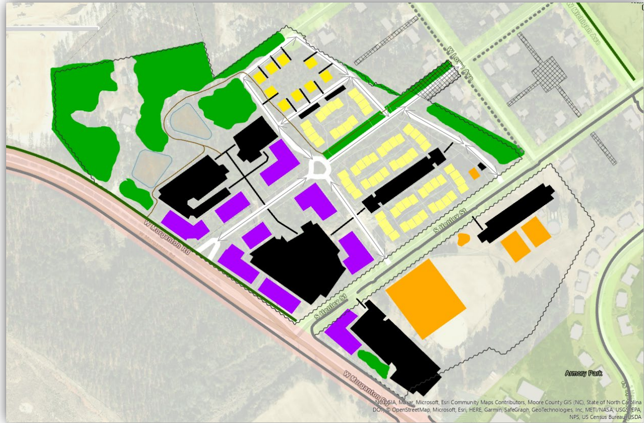
Figure 15. Conceptual Transportation Plan. The project boundary is shown in a waved border pattern. New paved roads are shown in white; driveways and parking are shown in black; existing sidewalks are shown in thick grey lines and the town's proposed sidewalks are in thick grey dashed lines (note that these are not proposed as part of this conceptual development plan); project sidewalks are shown in thin white lines; shared use trails are shown as brown lines; and stormwater management facilities are shown in light brown with blue waterlines. The double arrows represent two-way traffic while the single arrows represent one-way traffic.
