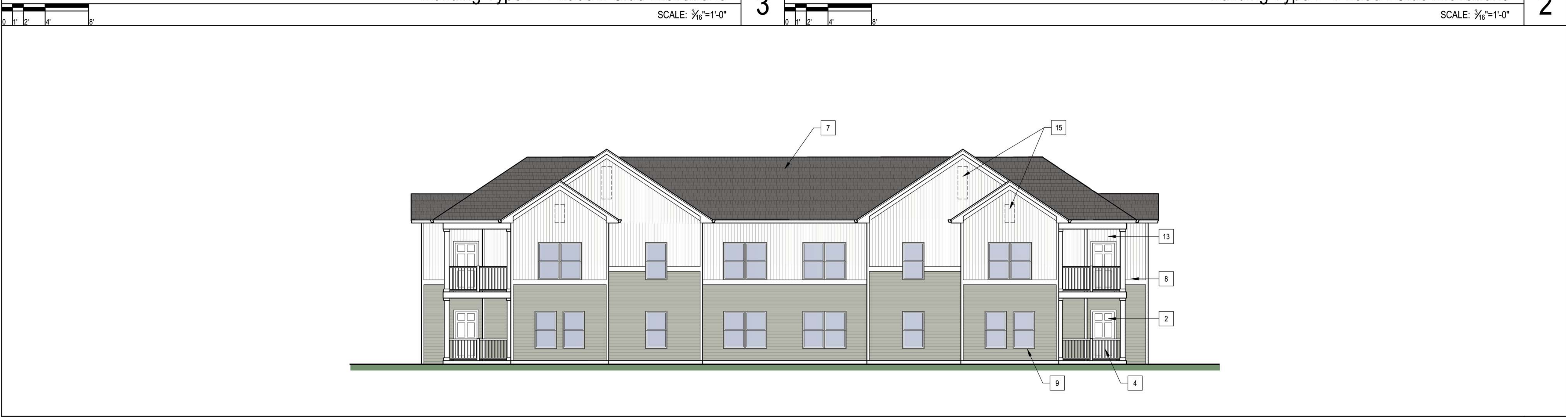
Building Type I - Phase I Front/Rear Elevations
