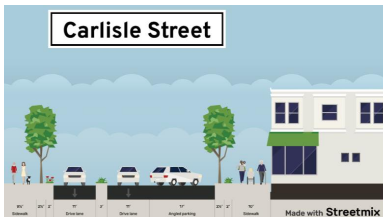
Figure 7: Planned Cross-section of Carlisle Street
