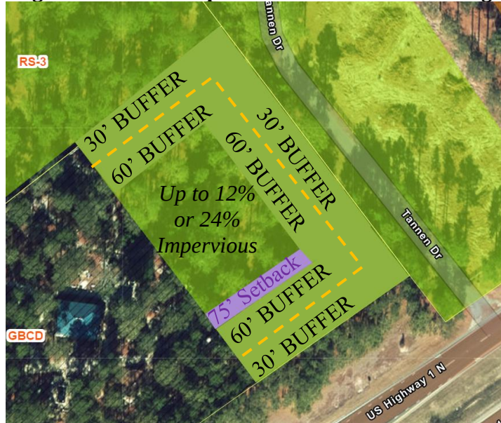
Figure 4: Buffer Requirements for Outside Storage
